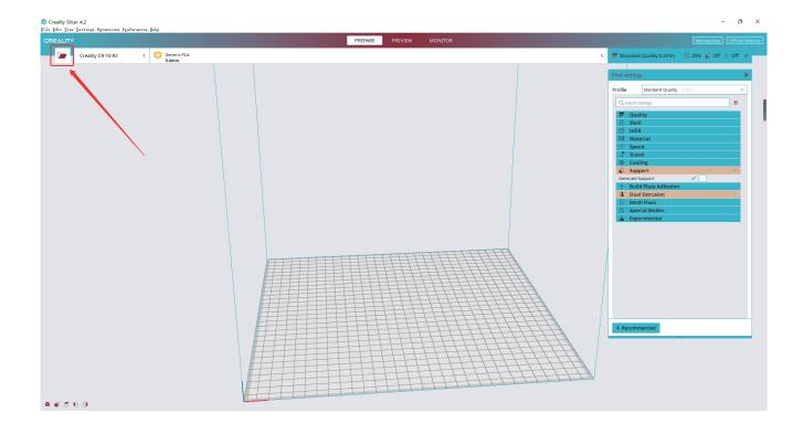
Method 3: Directly drag STL, 3MF, AMF or OBJ files to the printing platform.
