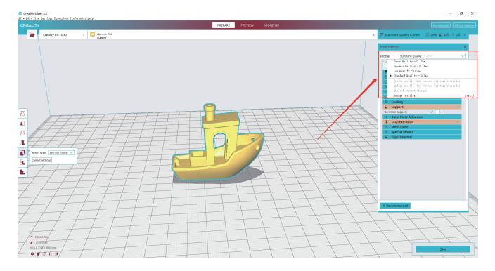
2. Specific print parameters include quality, shell, infilling and movement, etc.
